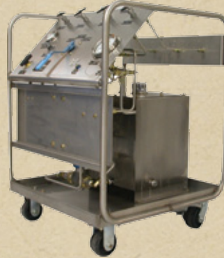
Mobile hydraulic or skydrol cart on casters with control panel for pressure testing valves, motors and various aircraft components.
